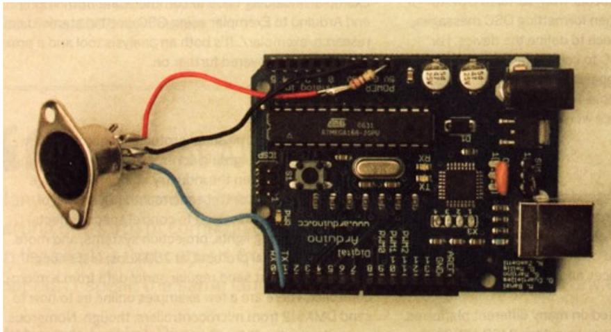
**NOTE:** Unplug MIDI cable when uploading programs (D1 is the TX part of the serial communication to the Arduino IDE).
