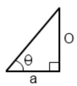
The arc-tan can compute the angle given the sides of a triangle:
